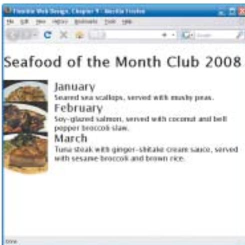
FIGURE 9.15 Floating the text elements to the right allows the images to sit beside the headings, but the list items will not expand to hold the full height of the thumbnails when everything inside the list items is floated.
