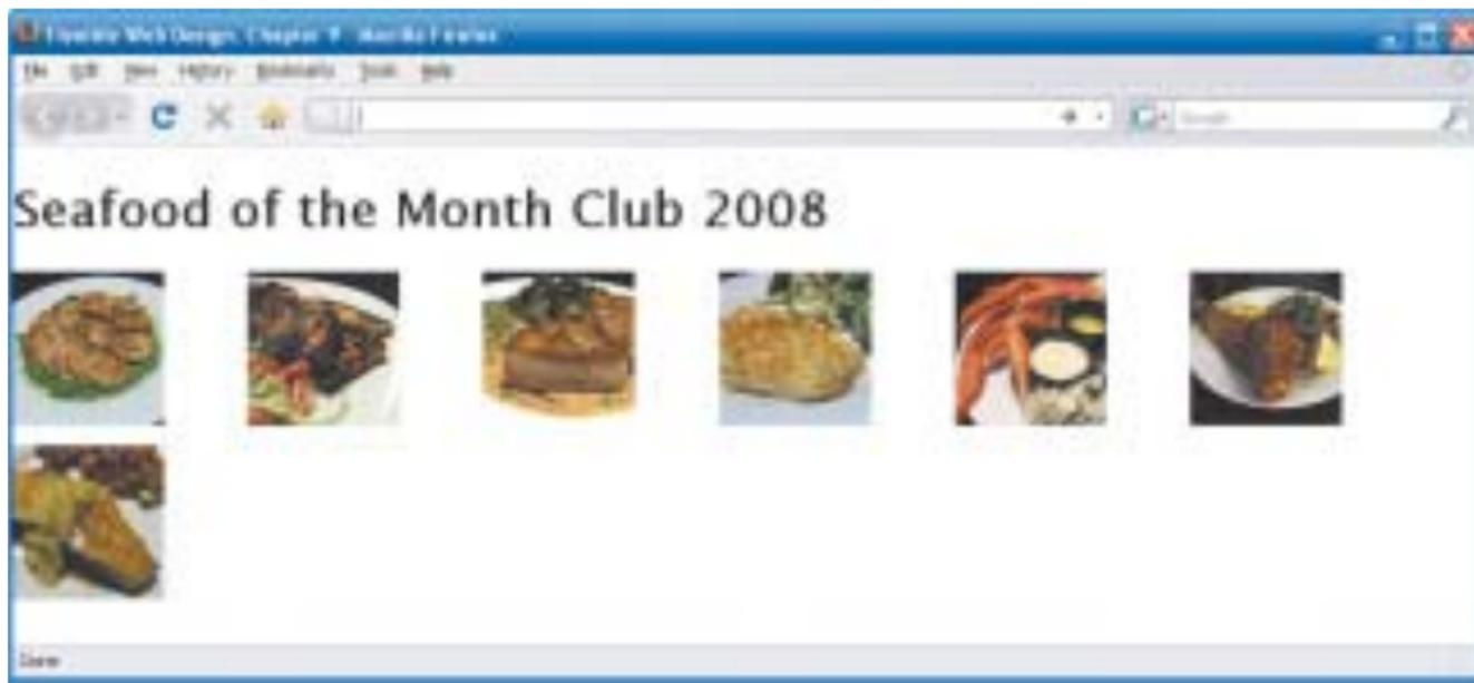
**FIGURE 9.21** Once the thumbnails reach their maximum widths, they will stop scaling, but will still adjust to the viewport size by moving farther apart to fill the space.
