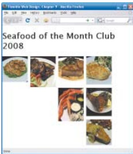
**FIGURE 9.18** The extra height on the second thumbnail blocks the fifth thumbnail from moving all the way to the left, leaving a gap in the second row. The same problem happens in the third row.
